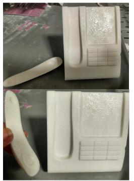
Fig 10 -Prototype after post processing with Color Bond
