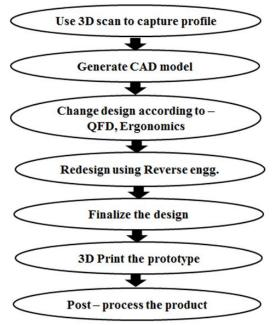
Fig 1- A logical structured approach has been taken to convert the scanned data points into desired features.
