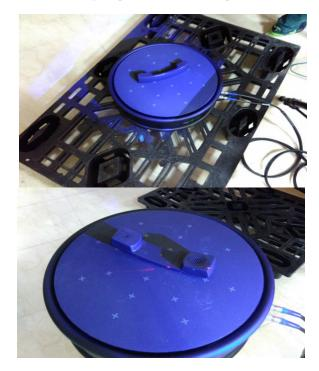
Fig 2-Scanning the receiver from different views for the registration by using structured light
