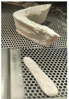
Fig 9 - Prototype of the base and receiver before cleaning and post-processing
